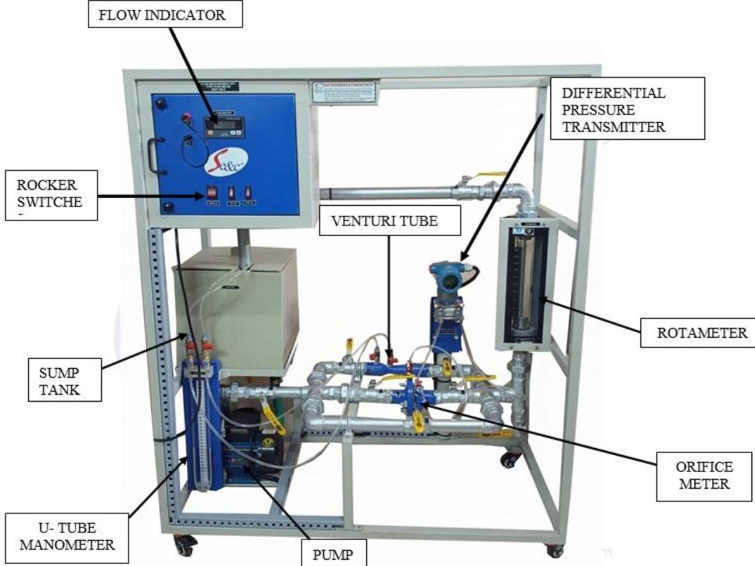
The **Setup for Calibration of Flow Sensor (SAP – 15D-I)** gives an idea regarding Flow Sensor & Flow Transmitter Principle. It outlines the procedure for calibration of flow Sensors/Transmitters.
